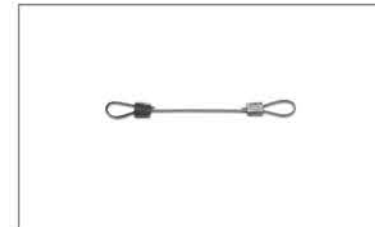
LAMP COVER SAFETY BELT ( 1340700008 ) DIAMETER: 0.6mm, LENGTH: 50mm, TENSION: 0.13kN, CANN' T SNAP THE STEEL WIRE ON EACH END OF CIRCLE SUITABLE FOR: ALL FIXTURES OF YAJIANG
