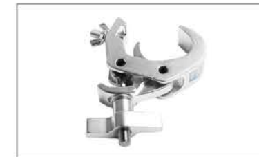
CLAMP ( X50081 ) AVAILABLE PIPE: 40-52mm MAX LOAD: 200KG SUITABLE FOR: PLUTO SS636XCE, SS646XCE, SS656XCE SS657SC HD, SS658SC, SS659SC SS660SC, SS661SC, SS662SC, SS663SC SS664SC CYAN SS631XCE, SS644XCE NEPTUNE SS671XCEM, SS673SCM, SS676SCM
